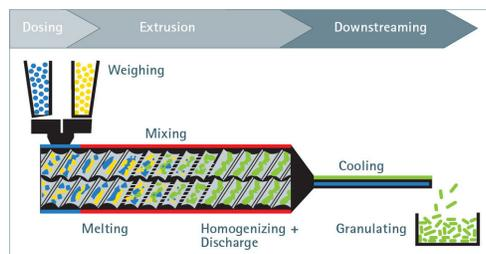
**Figure: Hot melt extrusion**
